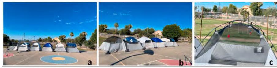
Fig. 1. Experimental setup of 6 identical tents, shown from left to right with different cover materials, as follows: control (no cover), mylar rescue blanket, white bedsheet, tarp, sunbrella fabric, and aluminum foil on cardboard. a: The Kestrel Heat Stress Meter (far left) on the tripod can be seen alongside the six tents. b: Side view of the six tents. c: Set up of Kestrel Drop sensors within the tents.
